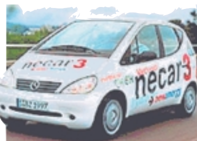
Photo 3: In its fuel cell car N-car 3, Mercedes uses methanol as its source for hydrogen for the fuel cell. Photo courtesy of Mercedes Benz.
