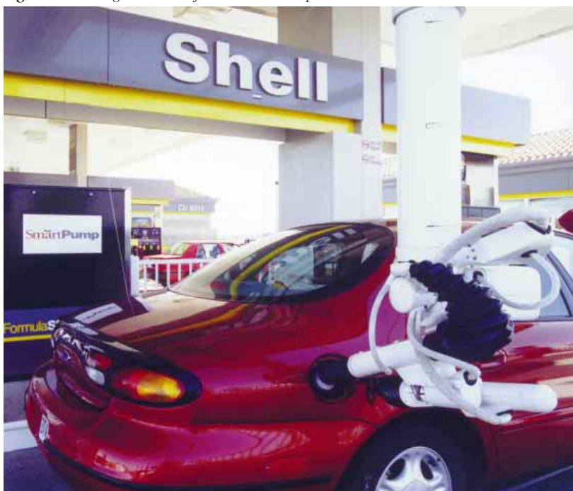
Figure 5 Fueling arm detail of Shell's Smart Pump
